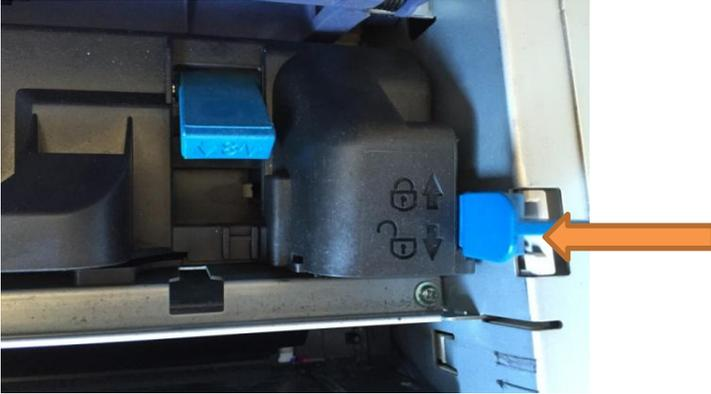
Remove fuser by gently pulling upwards using the handle
