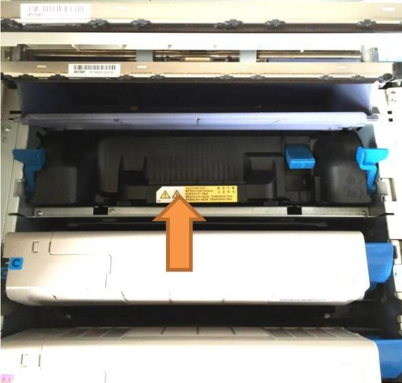
Unlock the fuser as indicated (left & right sides)
