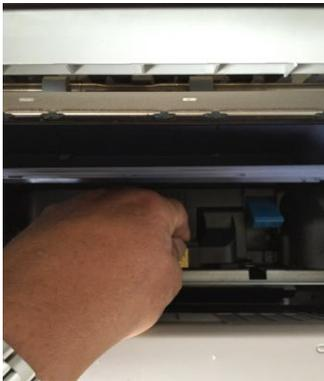
Replace the fuser with the new unit supplied and reverse the process detailed above (Don't forget to lock the fuser back in position!)
