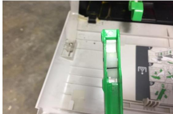
7: Insert "Wand" into the opening in drum
