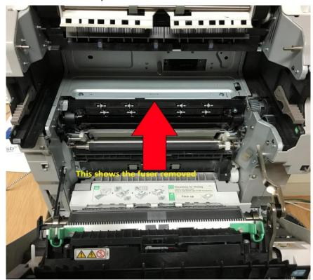
5: Insert new fuser and ensure that you lock it into place by pushing the two levers down..now close the front
